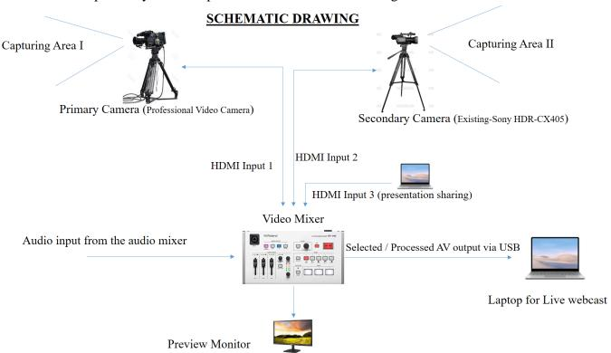
**Note: Custom made audio cable** to be provided for connecting the audio input from the audio mixer to the proposed Video mixer.
