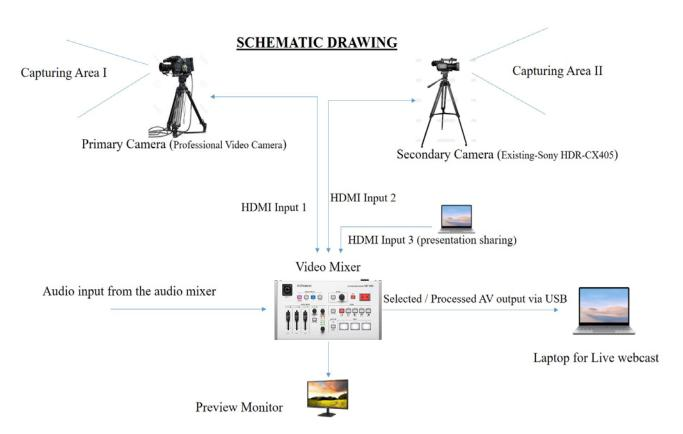
**Note: Custom made audio cable** to be provided for connecting the audio input from the audio mixer to the proposed Video mixer.
